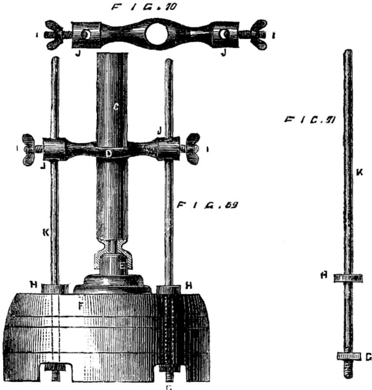
Fig. 69. *c*, gerd case; *d*, metal band to support the case; *ij*, supports for band, with hole for steel rods, *kkk*; *h*, base of rod, resting on the upper part of lower part of rod, with nut and thread to fasten them to the block, dotted lines showing the lower part passing through the block; *i*, thumb screws for fixing the block; *e* and *f*, block and nipple. Fig. 70. Band removed from the upright. Fig. 71. Rods (or uprights) removed from the band and block.
