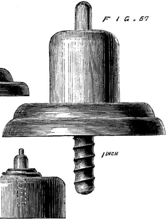
Fig. 60. Diagram of paper for 2oz. gerb, and 1oz. brilliant fire cases. Fig. 61. Diagram of board for 2oz. gerb cases. Fig. 62. Diagram of board for 1oz. brilliant cases. Fig. 63. Priming tool. Fig. 64. 1oz. nipple. Fig. 65. 2oz. nipple. Fig. 66. 1/2 lb. nipple. Fig. 67. 3/4 lb. nipple. Fig. 68. Sketch of nipple attached to the block.
