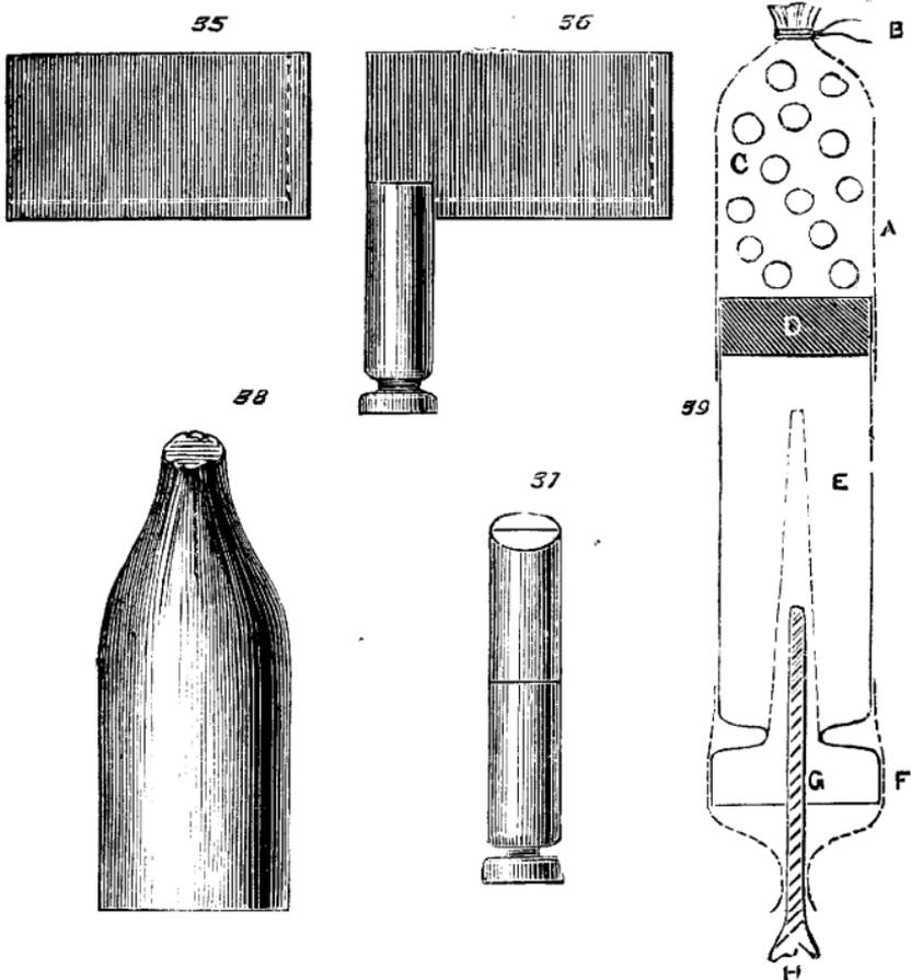
FIG. 39.—Finished rocket,  $\frac{1}{2}$ lb. size; A, rocket cap; B, top tied with string; C, stars; D, composition to ignite the stars and burst the cap; E, rocket case; F, blue cap paper for quick-match; G, quick-match; H, igniting point of rocket.
