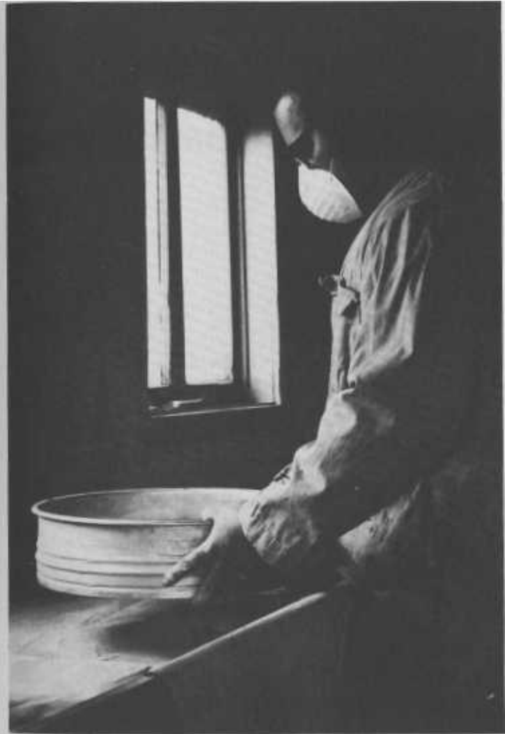
A pyrotechnician cautiously mixes a composition through a sieve to achieve homogeneity. Eye and respiratory protection are worn, and great care is taken throughout this critical phase of the manufacturing process. Sensitive compositions, as well as large quantities of any pyrotechnic mixture, should be blended remotely. (Fireworks by Grucci)
