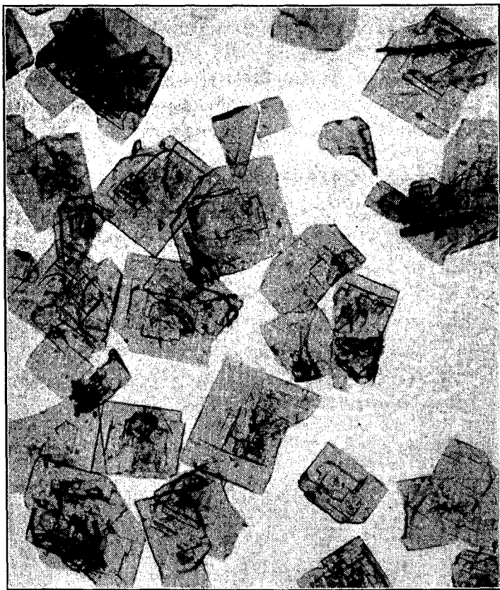
FIGURE 103. Diazodinitrophenol Crystals (90 \times ).
