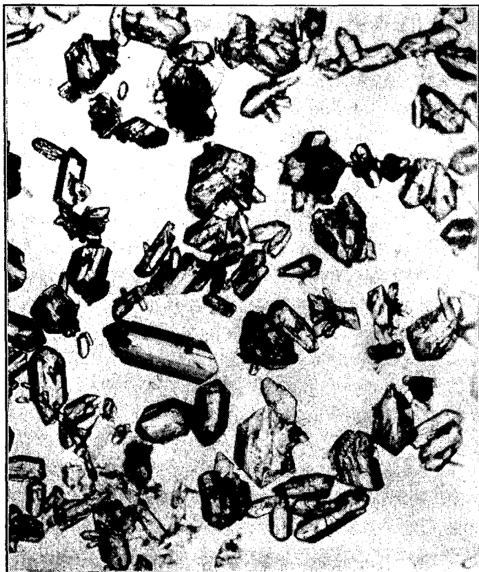
FIGURE 102. Lead Styphnate Crystals (90X).
