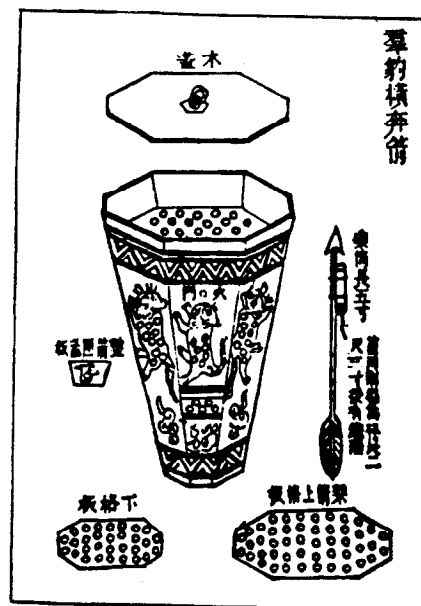
Fig. 4. The portable launcher above fired 40 rockets to a distance of 400 feet.
