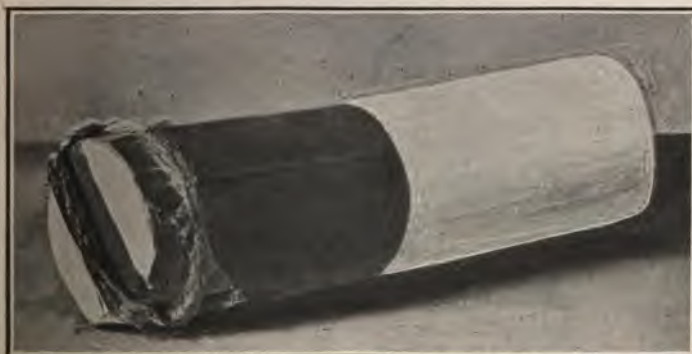
FIG. 49.—Wrapped briquette showing quick match and knot socket.
