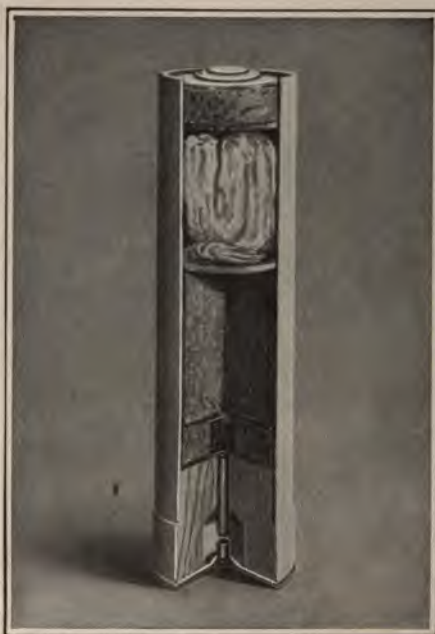
FIG. 133.—Sectional view of parachute rifle light.
