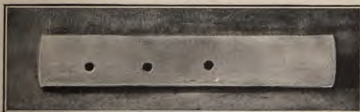
FIG. 34.—Smoke tracer showing vents.
