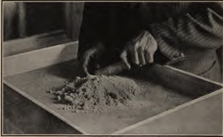
FIG. 43.—Loading charge into mold.
