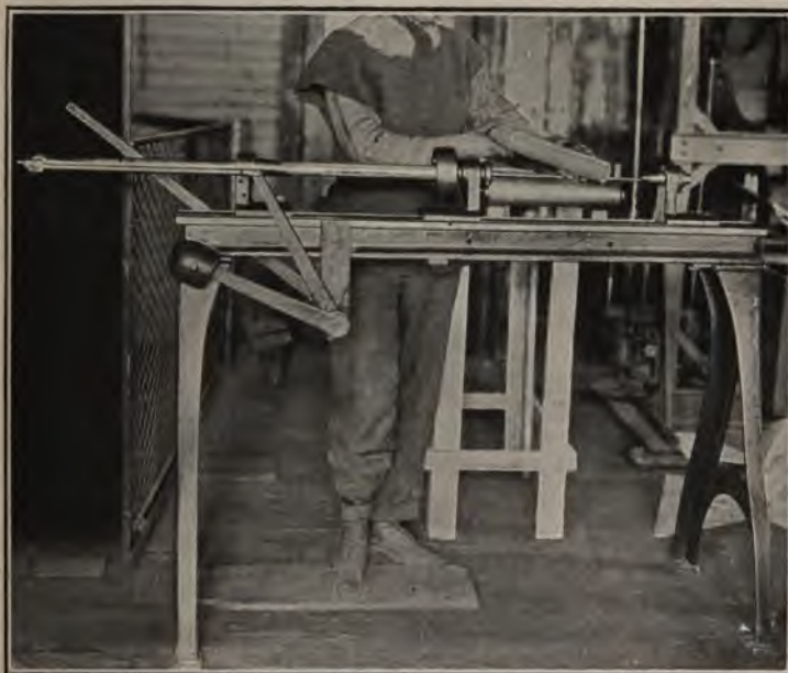
FIG. 9.—Case-rolling machine; removing case from machine.
