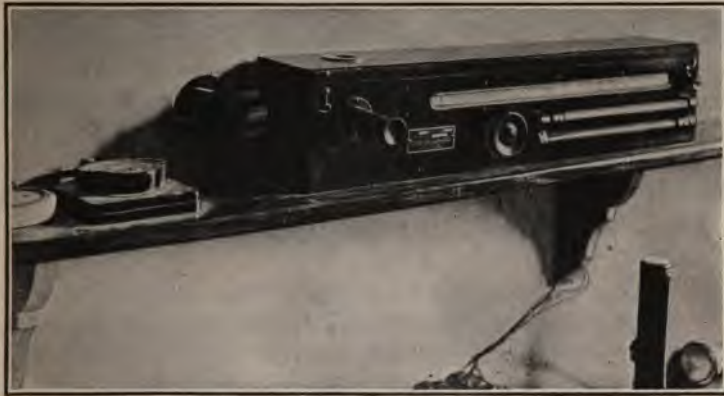
FIG. 211.—Standard photometer used in the Government testing laboratory.
