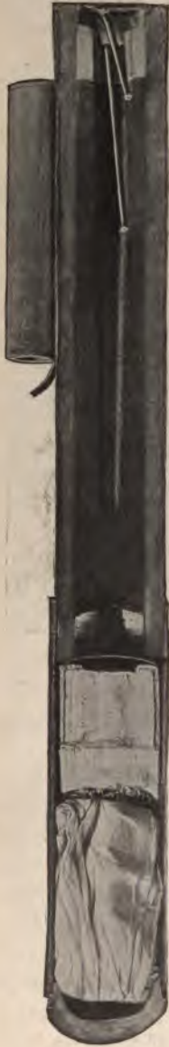
FIG. 39.—Cross-sectional view of completed rocket.
