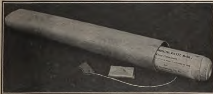
FIG. 71.—Placing rocket in wrapping carton.
