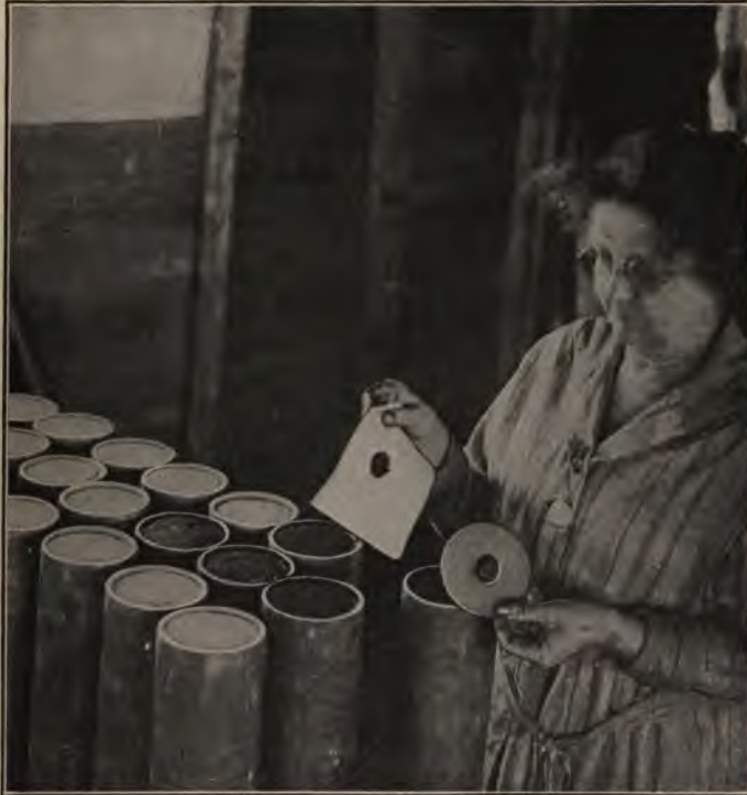
FIG. 106.—Assembling case bottom.
