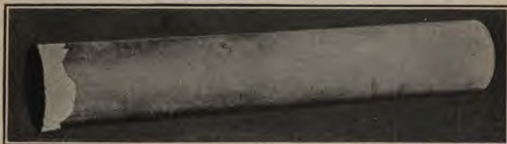
FIG. 26.—Rocket body showing drumhead and prime.
