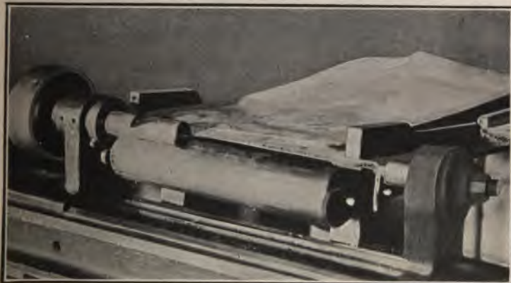
FIG. 4.—Case-rolling machine showing pasting notch.
