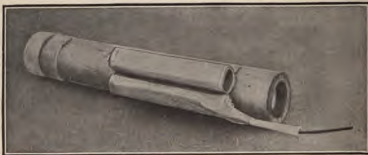
FIG. 37.—Rocket body showing smoke tracer attached
