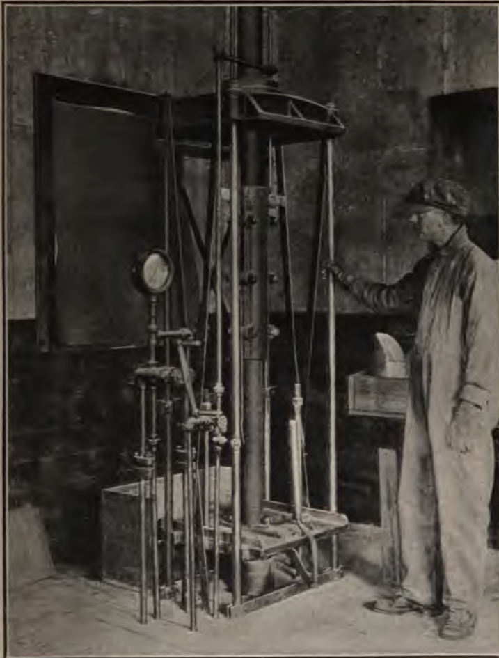
FIG. 98.—Hydraulic press ; removing jacket.
