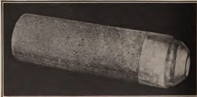
FIG. 68.—Rocket head showing band holding identification plug in position.
