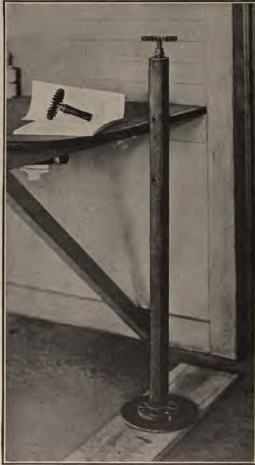
FIG. 123.—Apparatus for testing detonating caps.
