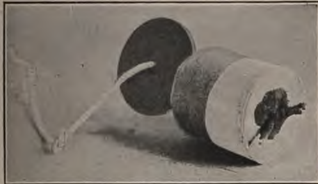
FIG. 146.—Quick match sealed with prime.
