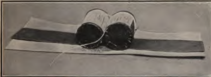
FIG. 188.—Lights on wrappers showing tearing cord.
