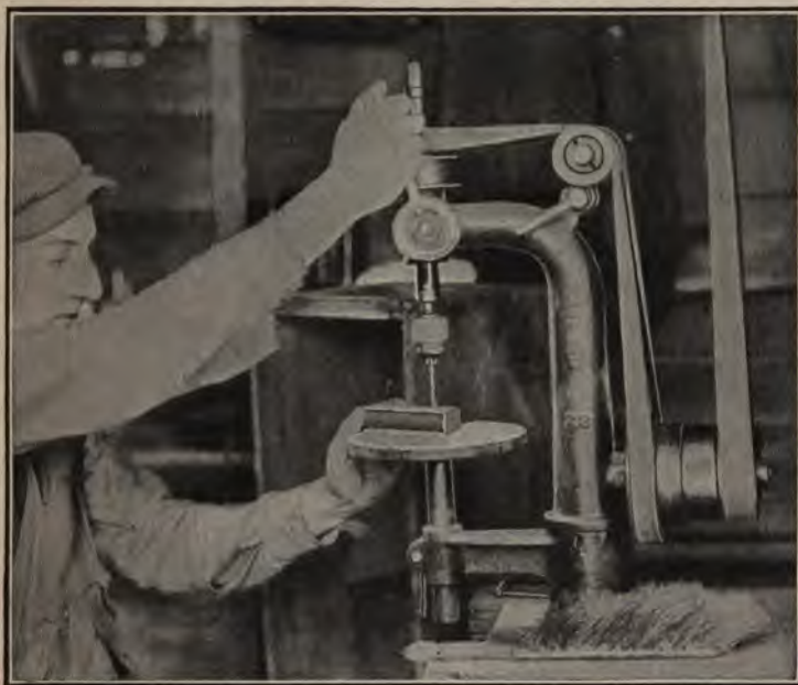
FIG. 33.—Drilling smoke tracer.
