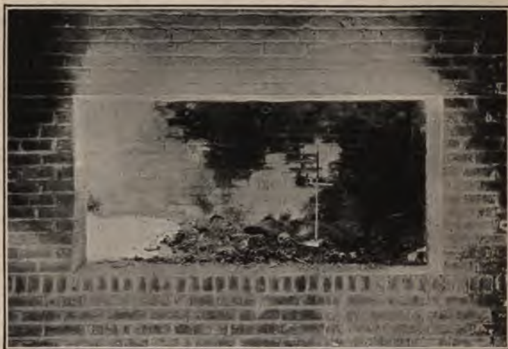
FIG. 216.—Fireproof chamber for testing samples.
