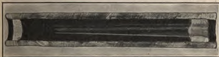
FIG. 17.—Sectional view of rocket body.
